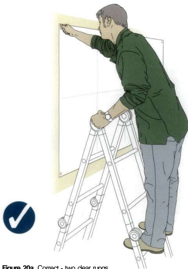
Figure 20a Correct - two clear rungs
