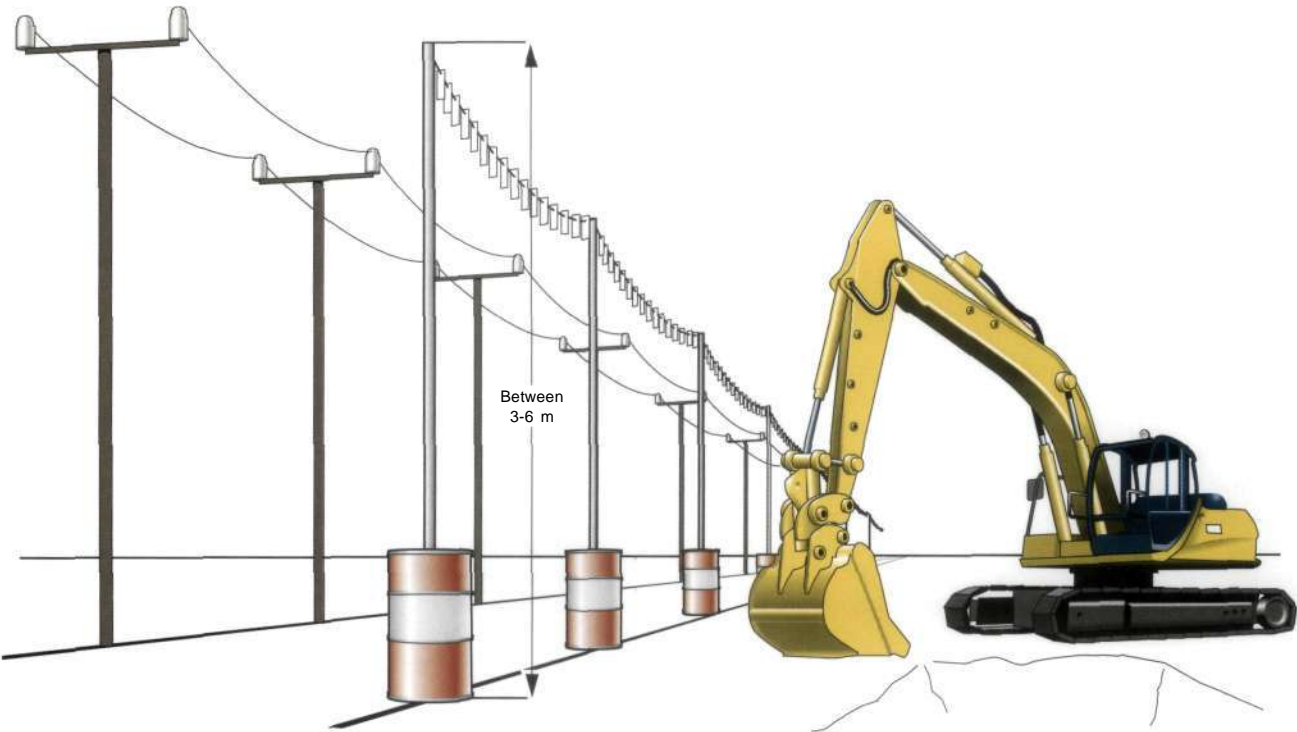
Figure 49 Ground-level barrier for plant working near an overhead power line
