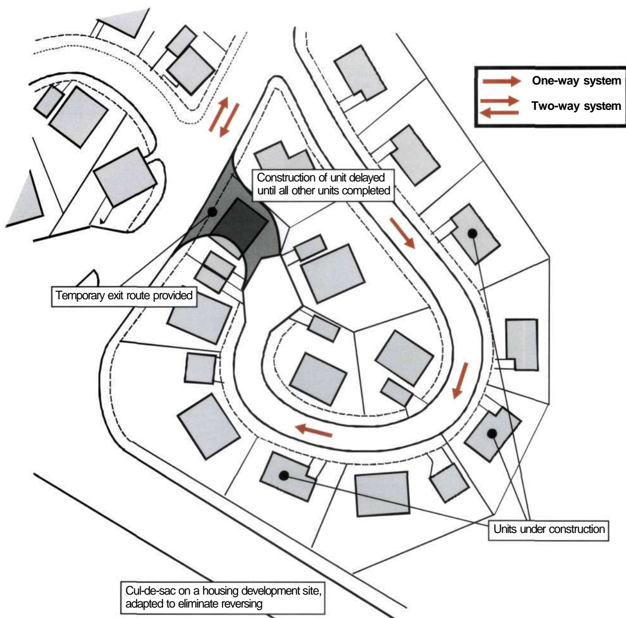
Figure 32 Provide drive-in/drive-out access to delivery and work areas
