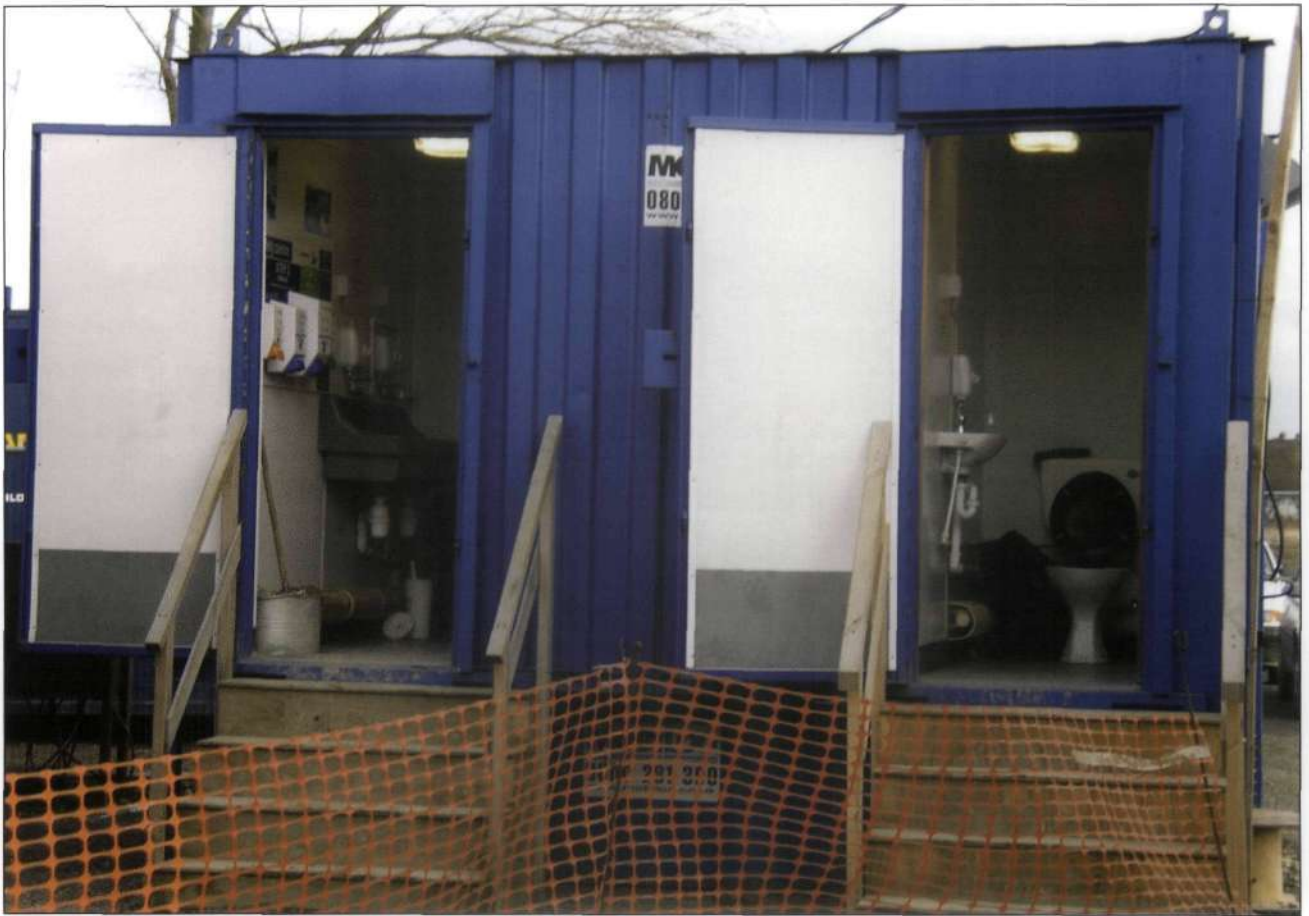
Figure 2 A self-contained water-flushing toilet block with built-in tank
