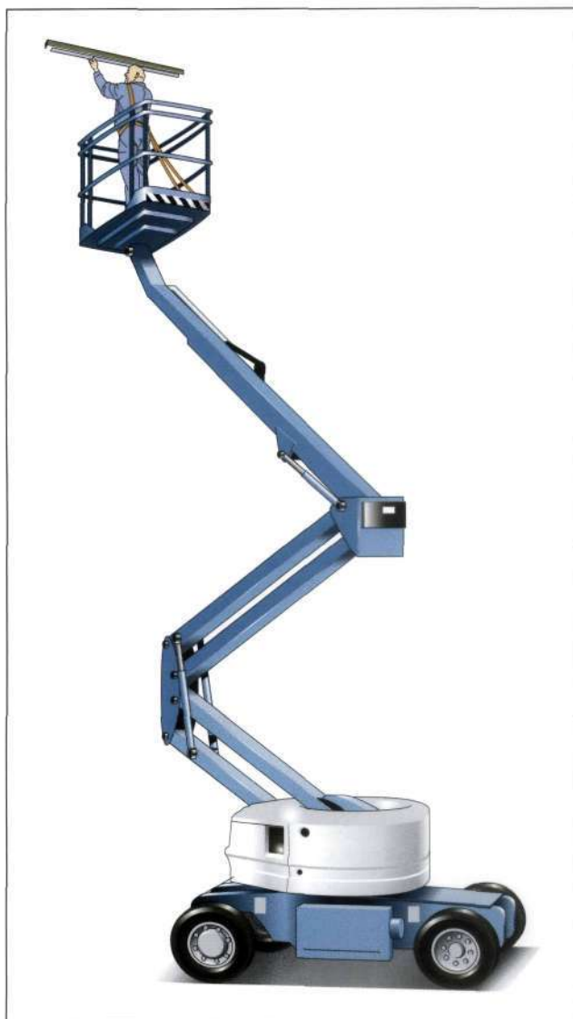
Figure 13 A mobile elevating work platform
